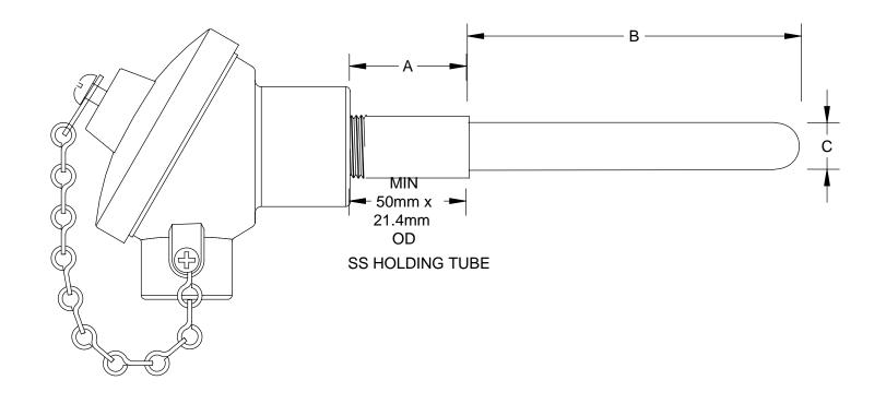
TYPE R, B, N AND K THERMOCOUPLES **SMALL ALUMINIUM HEAD IP65** COMPLETE WITH CERAMIC SHEATH HIGH TEMPERATURE
